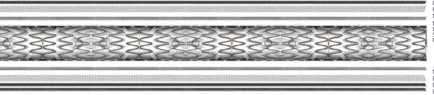
Resinated Pad Polyester Pad Protective Mesh Mid-Section Support Pad 12.75 Gauge Steel Offset Innerspring w/Double Edge Side Supports (12 on Twin and Full. 14 on Queen and King)
