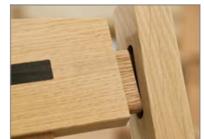
Precision cut mortise and tenon joints ensure solid, durable structural integrity.
