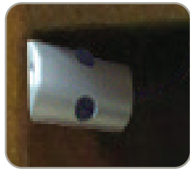
SENSOR TURNS LIGHTS ON WHEN DOOR OPENS
