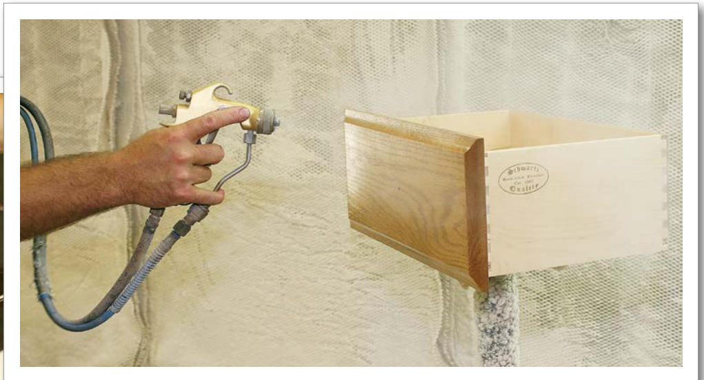
The sealer and top coat are carefully applied, giving each piece a smooth and durable finish.
