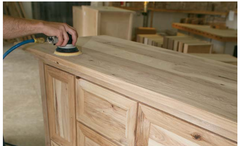
Each piece is hand sanded, preparing it to be finished.
