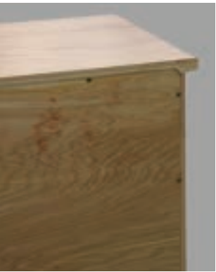
Inset Backs with Screw Fasteners
